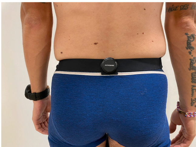
Fig. 1. The Movesense inertial measurement unit attached to the sacrum of a representative participant using an elastic strap belt.
